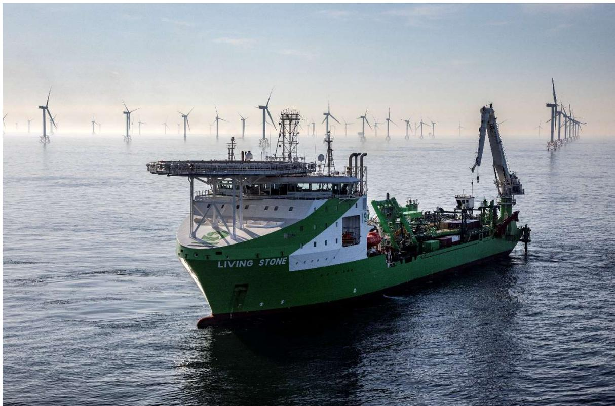
**Image caption:** DEME Offshore’s cable installation vessel ‘Living Stone’ will be deployed to lay the 650km of 66kV inter-array cables and associated cable protection systems for Dogger Bank A and Dogger Bank B. **Image source:** DEME Offshore
